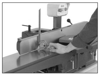
Figure 49. Adjusting fence to 90°.
